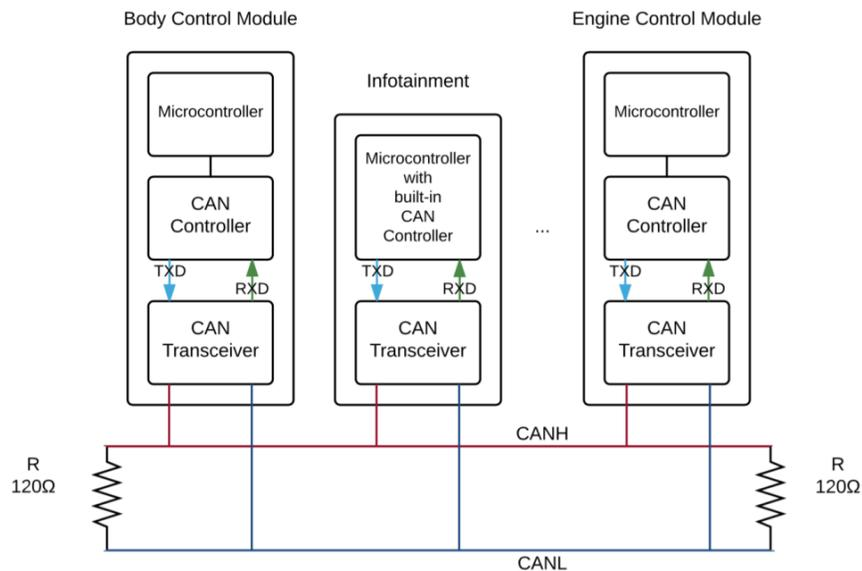
Figure 2: Typical CAN-based in-vehicle network (top) and how it's electrically connected to the CAN bus (bottom). The Microcontroller implements the "application" logic, the CAN Controller implements the CAN logic, and the CAN Transceiver is responsible for translating logical "zeros" and "ones" into electrical signals.
