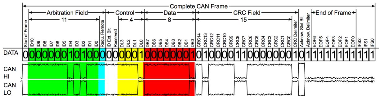
Figure 3: Structure of a CAN frame (source: Wikipedia - [https://en.wikipedia.org/wiki/CAN\\_bus](https://en.wikipedia.org/wiki/CAN_bus))
