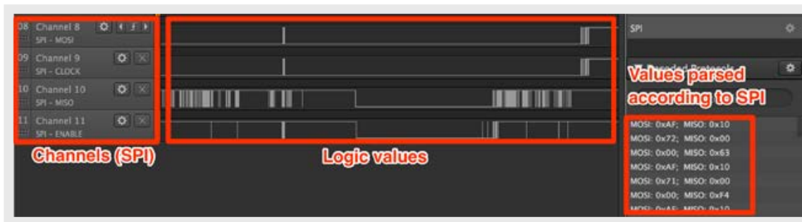
Figure 34. Output of the logic analyzer (bottom right) while tapping on the SPI bus
